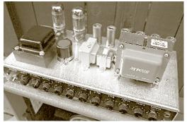
chassis sizes: CH1. 15" width w/four 9 pin sockets and two 8 pin sockets, transformers up to the 50 watt size.
