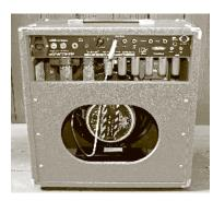
One of our favorite features is the 50 watt/40 watt switch on the back panel that changes the bias from fixed to cathode for a completely different feel. With the 40 watt cathode biased setting you can also change the 6L6 output tubes to 6V6s,
