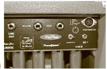
Coil setting sets the amount of bass gain in the input stage, relieving you of perhaps resetting EQ when switching from single coils to humbuckers.
