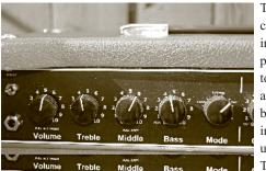
The Volume control includes a pull switch to engage a midrange boost that increases upper mids. The Middle
