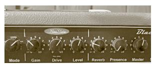
This is where you mine and manage overdriven tones and distortion. The Gain control can be bypassed by clicking fully left, otherwise, you're setting the amount of signal being sent to the first gain stage, which produces variable levels of
