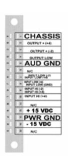
Note: On the Tube EQ (Pin 15) is connected to 48v and must be used for the tube EQ to operate
